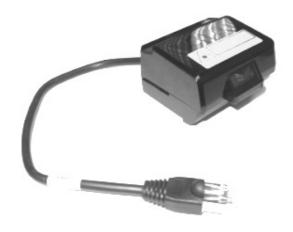
The laser of the 1D barcode reader is directed downward and can be activated by proximity sensor when any object is place within its range. At the closest point, it has the ability to scan up to 44mm wide at an angle of 44°.
