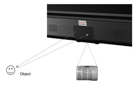
The range of the distance to read a barcode is dependence on the resolution of the barcode to be scanned. Please refer to the following chart for a quick reference.
